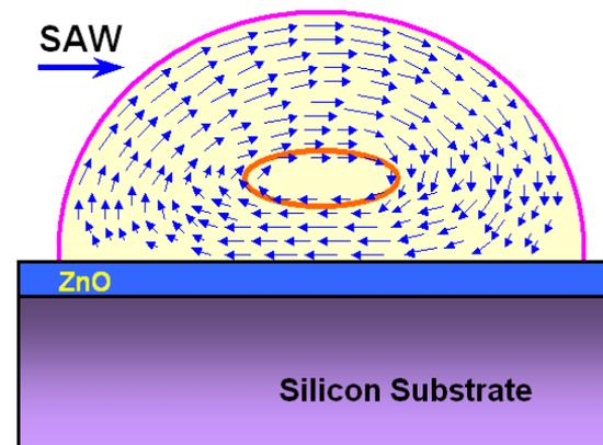
Schematic drawing of mixing patterns
