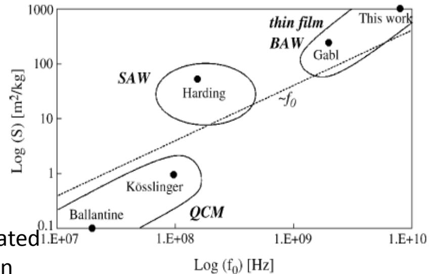
Comparison of sensitivity of acoustic wave devices
