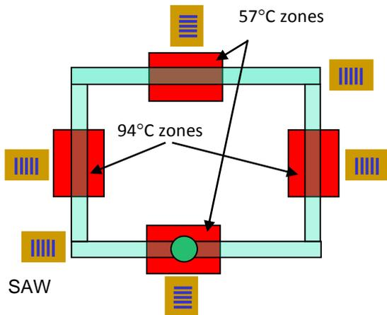
SAW based Lab-on-a-chip
