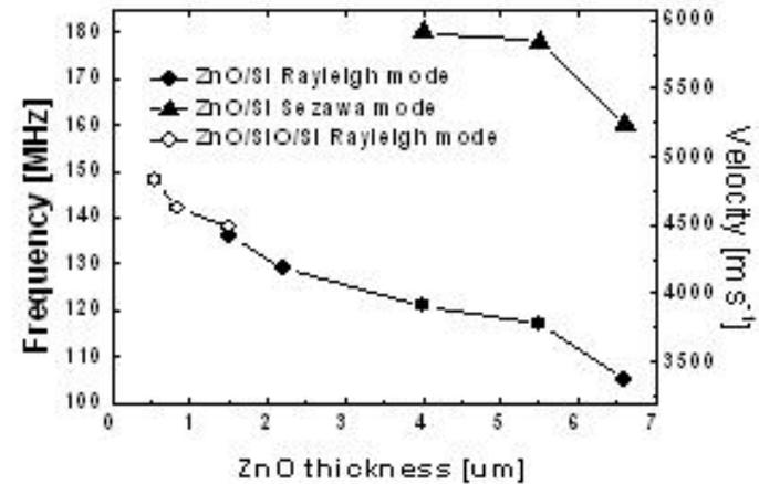
SAW frequency vs. film thickness
