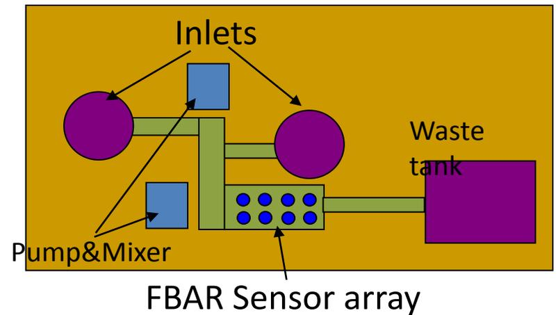
Acoustic wave-based lab-on-a-chip
